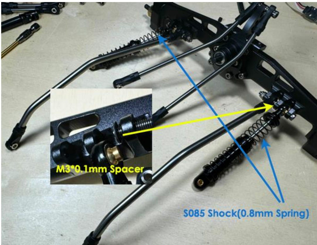
Assembled Rear lower link and shock(0.8mm spring) to Rear axles:
