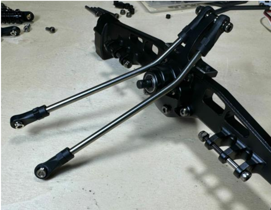
Assembled Rear lower link and shock(0.8mm spring) to Rear axles:
