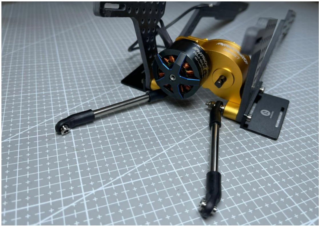
Step9: Assemble Rear lower link to Rear Axles:
