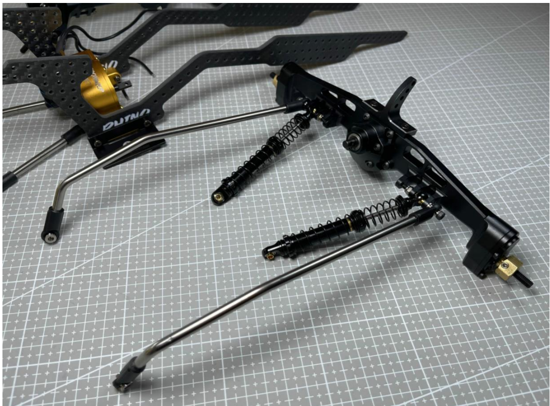
Step9: Assemble Rear lower link to Rear Axles:
