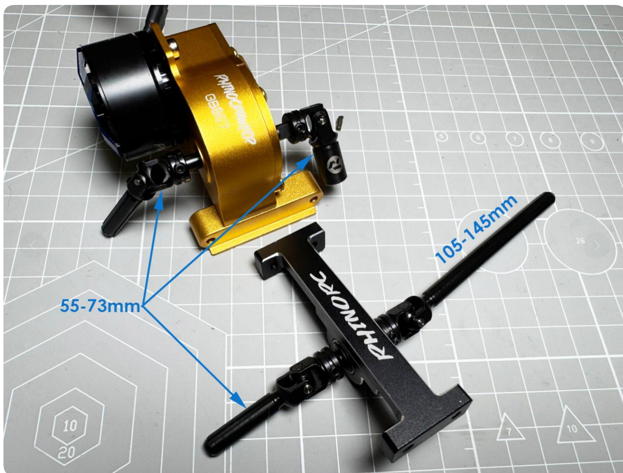
Assemble front upper links and servo mount
